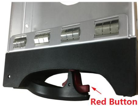
Figure 2-1 Opening the handle
